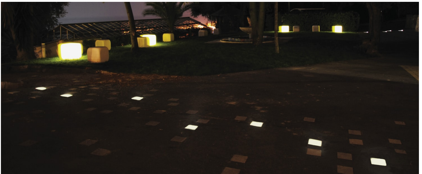
Landscaped garden. Creation by the artist Henri Olivier on an esplanade in the City of Menton. Luminous walkway with very low voltage embedded paving stones ECO-STONE99. Photography : Henri Olivier.
